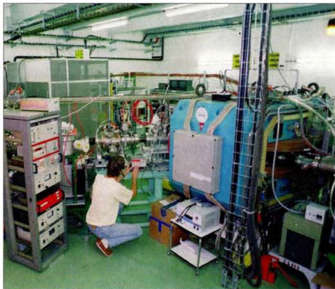
Measuring short-lived isotopes – the MISTRAL radiofrequency spectrometer at CERN's ISOLDE.
