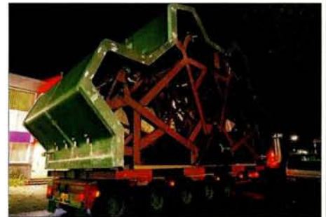
A half-shell of an ATLAS end-cap toroid arrives at Amersfoort for machining (Machine Fabriek Amersfoort).
