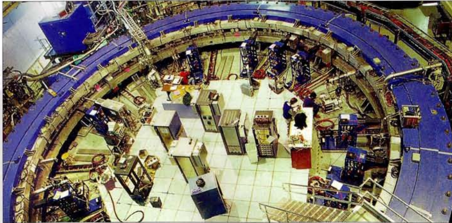
Above: precision masterpiece – the superconducting storage ring at Brookhaven used to measure the muon's magnetism. Right, top (left to right): Georges Charpak, Antonino Zichichi, Hans Sens, Francis Farley and Francis Müller, who performed a pioneer precision measurement of the muon's magnetism at CERN in 1961. Farley is one of the collaborators on the new Brookhaven experiment. Right, bottom: the microsecond wobbles in the spectrum of positrons from muon decay in Brookhaven's storage ring.
