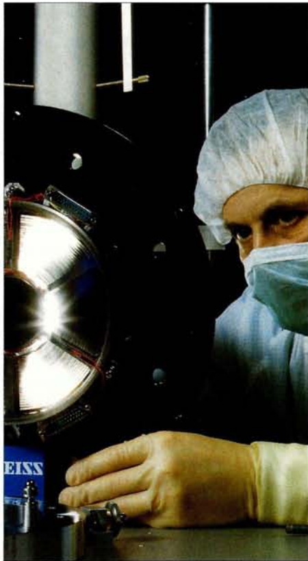
Additional axion optics – a spare X-ray lens module constructed for the ABRIXAS orbiting X-ray telescope. (Carl ZEISS/ Oberkochen-Germany.)
